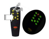
The rear (back) lighting allows for quick, easy identification of the keys even in low-light conditions: to light up the keyboard with the transmitter operational press the ON key and hold it down until the rear lamp comes on (signalled by two beeps). If the transmitter is off, prolong the pressure on the ON key until the rear lamp comes on.
