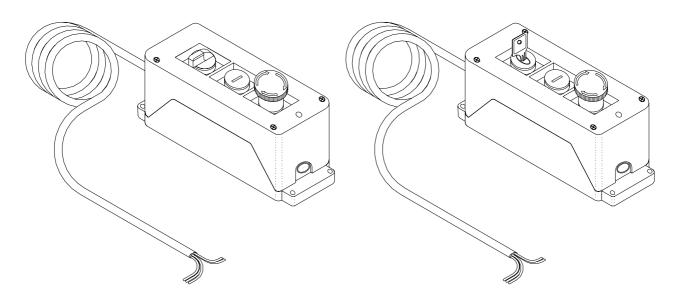
By means of the selector (supplied as optional) the outputs can be manually activated; the auxiliary is activated at the same time as the two outputs.
