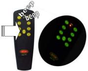
The rear lighting allows for quick, easy identification of the keys even in low-light conditions: to light up the keyboard with the transmitter operational press the ON key and hold it down until the rear lamp comes on (signalled by two beeps). If the transmitter is off, prolong the pressure on the ON key until the rear lamp comes on.
