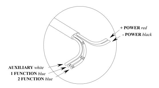
N.B. the 1, 2 and AUX functions, when activated have the same voltage as that of the power supply.
