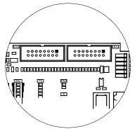
16 pole IDC connection (optional) to connect one or more expansion boards.
