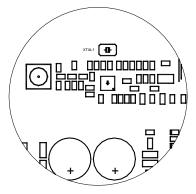
433MHz SUPERHETERODYNE FM/FSK receiver realized in SMT technology, in compliance with the EN 300 220 European standards.
