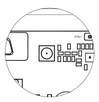
The receiver is supplied with an internal  $1/4 \lambda$  aerial with an SMA connection. If higher system performance is required the flexible aerial may be unscrewed and a vehicle aerial can be connected (see page 18).
