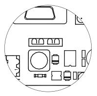
15A protective fuse (maximum) on output power supply line.
